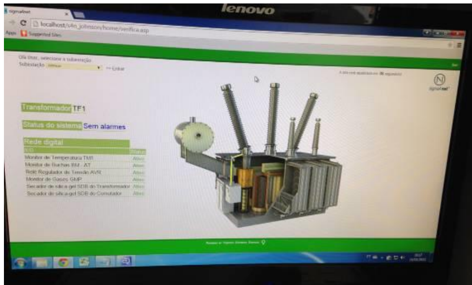
Fig. 08 - Monitoring software screen with the transformer failure graphic identification system.
