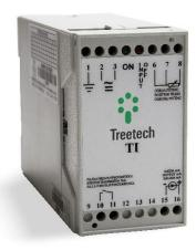
The Insulated Transducer (TI) is used in monitoring and protection systems for power transformers and reactors. Its function is to convert analog signals from temperature sensors (RTD), position of taps (potentiometric transmitters of on-lap tap changers), or current loop (signals in mA) into output values proportional to the input values. In the case of a RTD input, the TI performs the linearization of the sensor curve to obtain increased accuracy.
