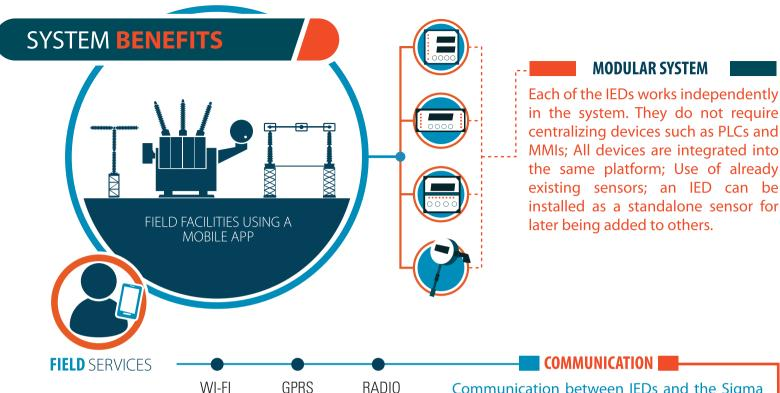
Communication between IEDs and the Sigma ECM® can be implemented by means of wireless technology (GPRS, Wi-Fi, Wi-Max, Radio), twisted pair or fiber optics.
