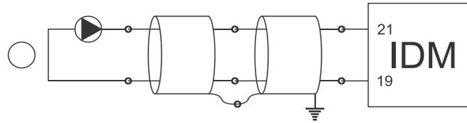
**Figure 19 – TAP position measurement through mA Analog Signal.**
