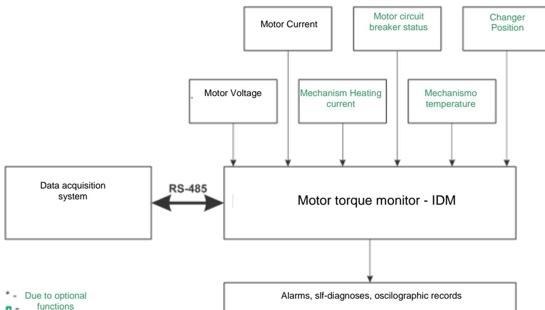
**Figure 2 – Composition of the Torque Monitoring System**
