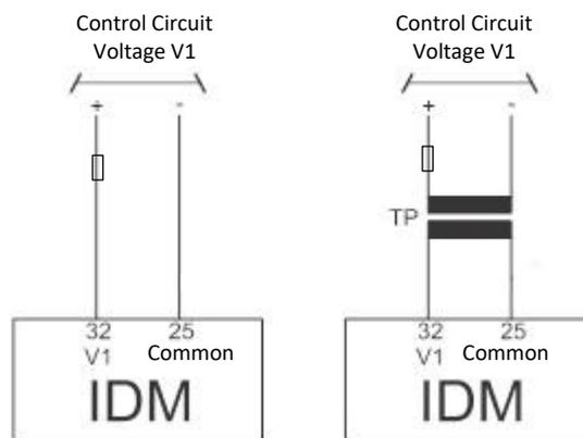
**Figure 11 – Connection to measure the voltage of the motor's control circuit without and with use of a PT.**
