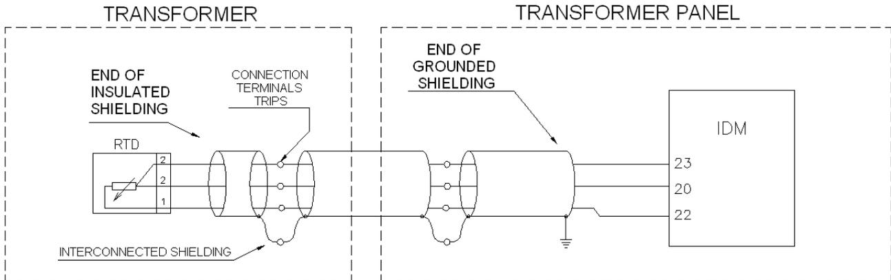
**Figure 20: Connection of the interconnection shielding between RTD sensors and the IDM**
