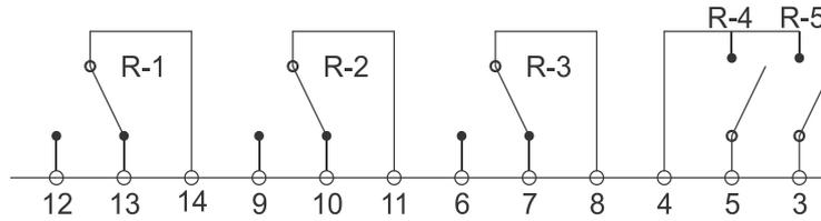
Figure 21 – IDM output relays
