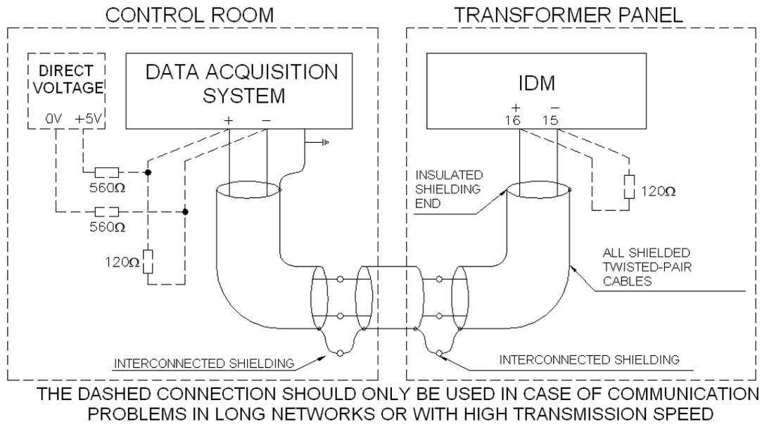
**Figure 7 - Connection and grounding of the shielding of the RS-485 serial communication**
