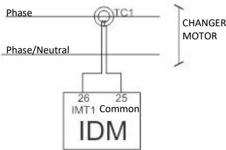
**Figure 12 – Measurement of supply current of an AC motor 1Φ.**
