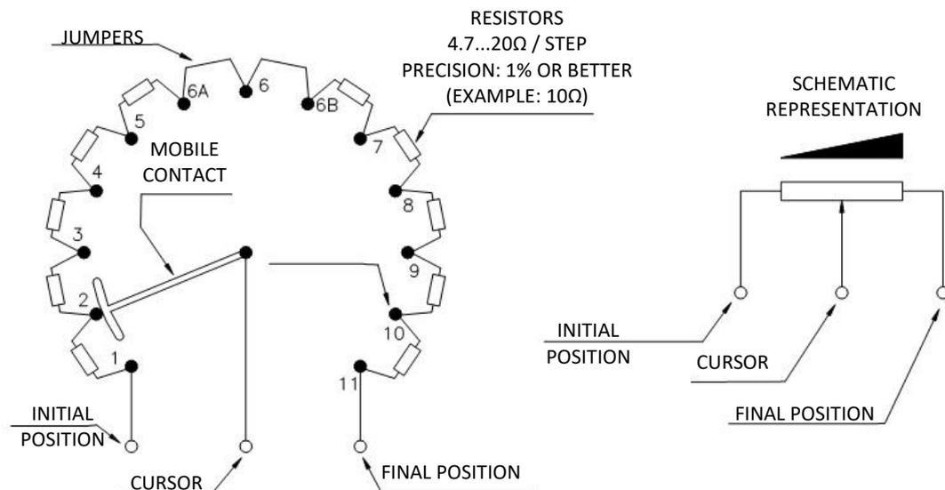
**Figure 18 - Configuration of the potentiometric transmitter's resistors in the intermediary positions of the on load tap changer**
