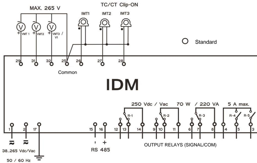
**Figure 6 - IDM input and output terminals in their standard configuration**
