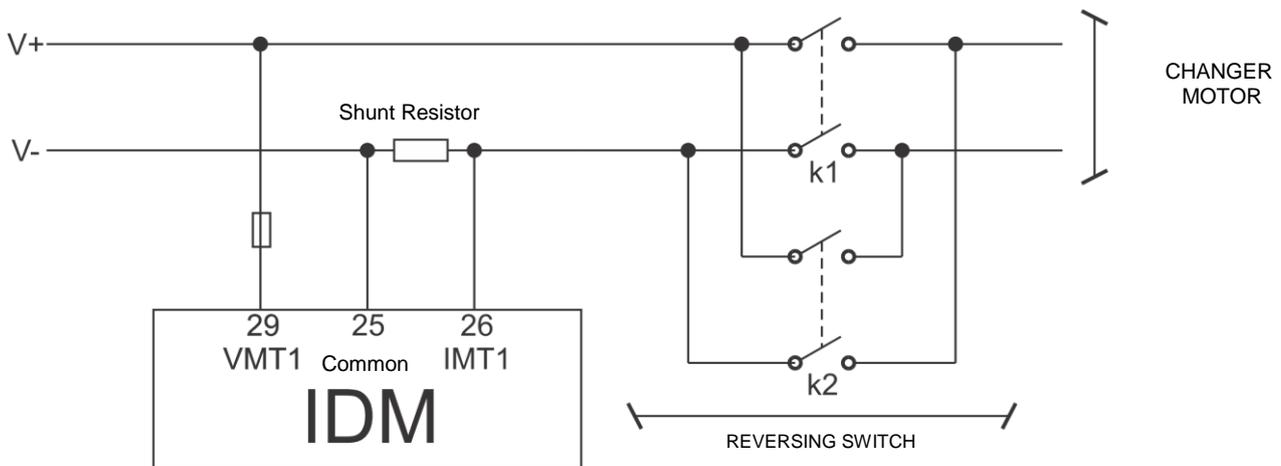
**Figure 8 – Voltage and current connection for DC motors.**
