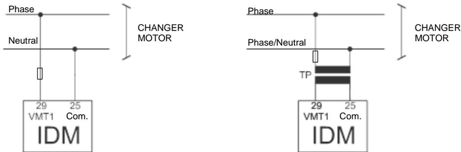
**Figure 9 – Voltage connection for single-phase AC motors without and with the aid of PT.**
