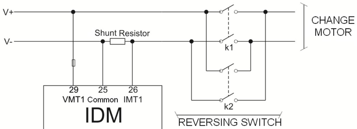
**Figure 14 – Voltage and current measurement connection from the DC motor to the IDM.**
