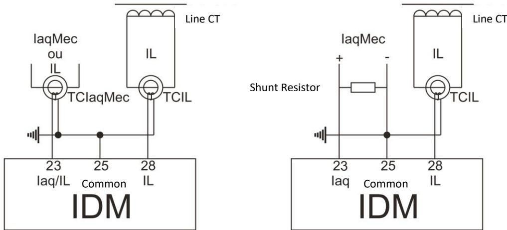
**Figure 15 – Diagram for measurement of the line and heating currents.**
