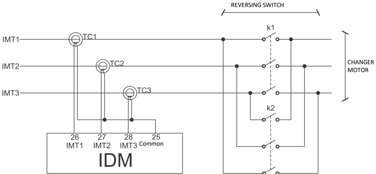
**Figure 13 – Electrical connection diagram to measure the currents.**
