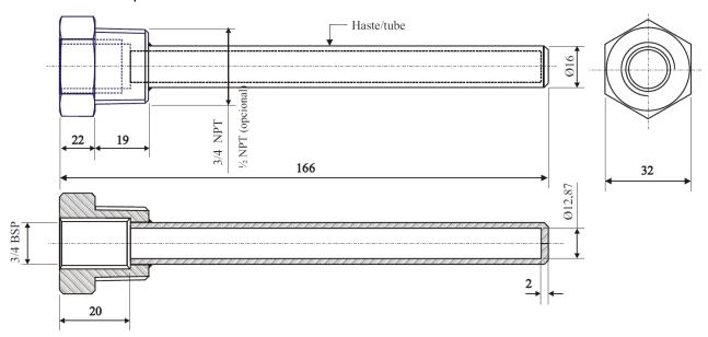
The wells are made of 304 stainless steel, a material very resistant to corrosion and very used as protection in temperatures up to 900 °C. The dimensions of the figure above are in mm.
