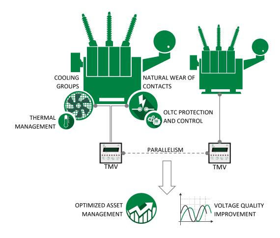
**Temperature Monitor and Voltage Regulator – TMV** typical application.
