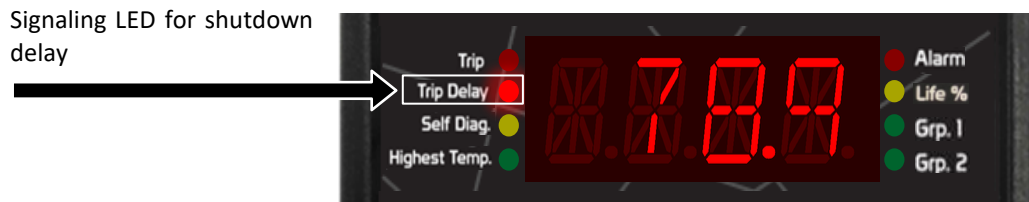
Figure 24 – Signaling LED for shutdown delay indication
