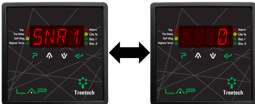
Figure 13 - Display indicating part 1 of the serial number
