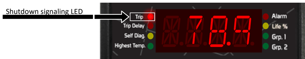
Figure 26 – Shutdown signaling LED
