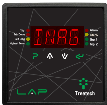
Figure 18 - Display indicating the active INAG option
