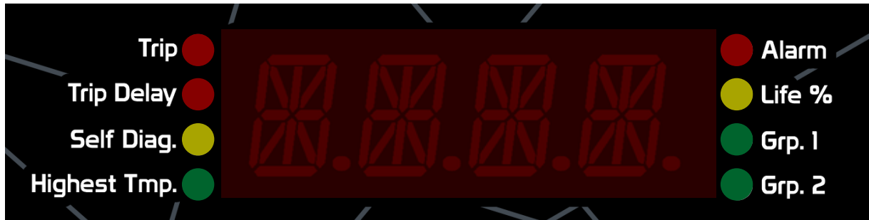
Figure 20 - LAP signaling LEDs
