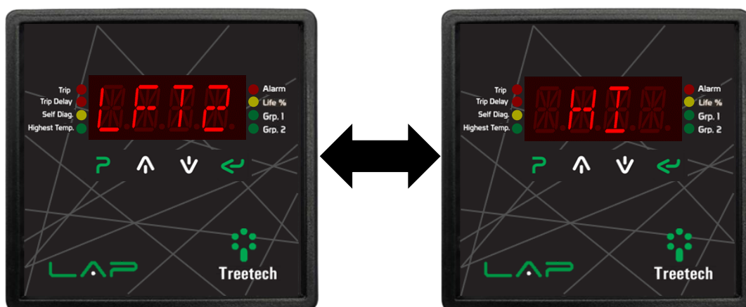
Figure 29 - Indication of lifetime greater than 50 years
