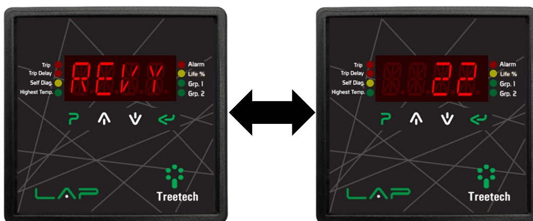
Figure 16 - Display indicating board revision year
