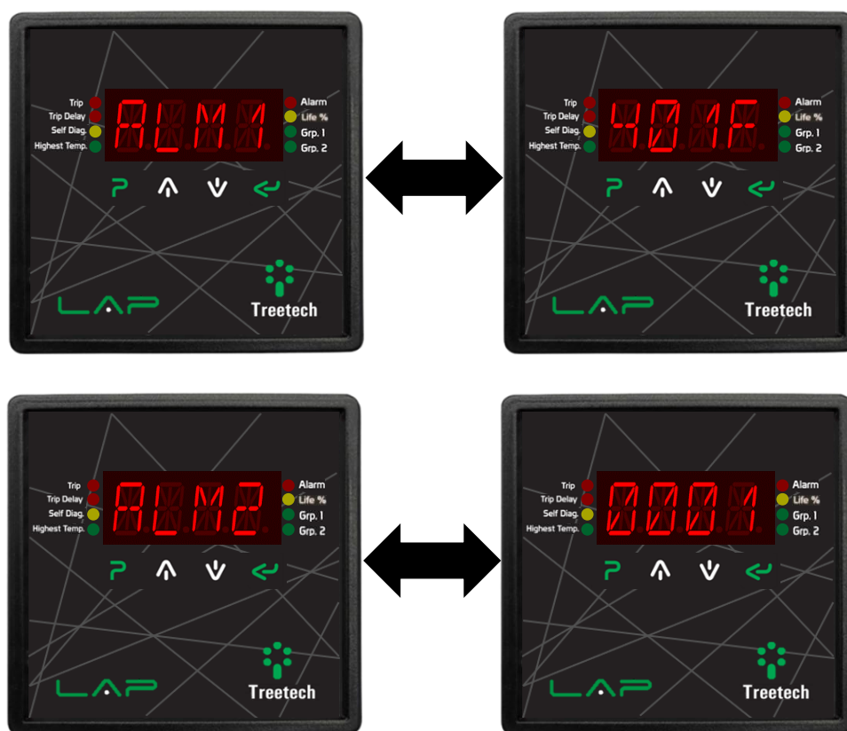
Figure 43 - Alarm memory query screens
