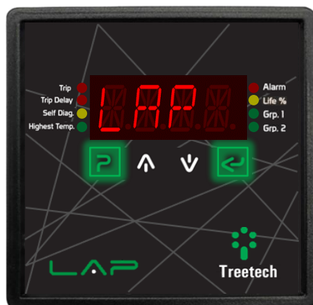
Figure 8 – Command to access equipment information
