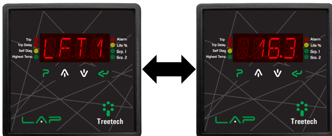
Figure 27 - Indication of lifetime, in years
