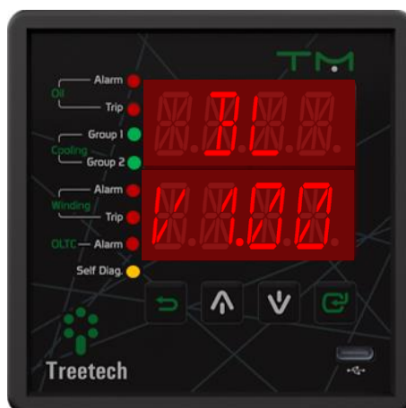
Figure 14 - Display indicating bootloader version
