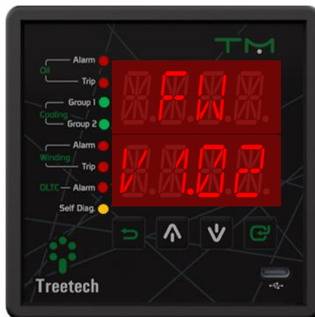
Figure 12 - Display indicating firmware version
