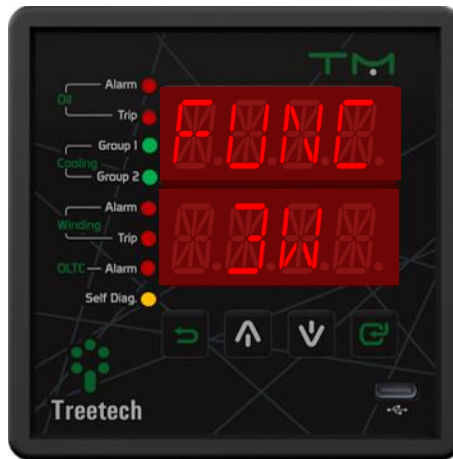
Figure 16 - Display indicating the number of windings
