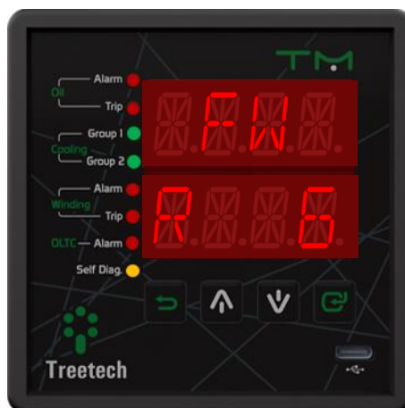
Figure 13 - Display indicating firmware release version
