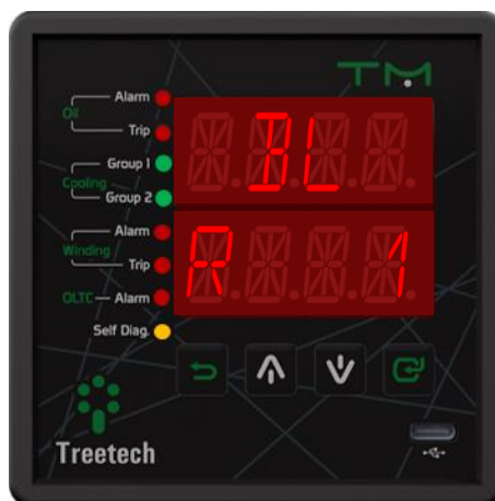
Figure 15 - Display indicating bootloader release version
