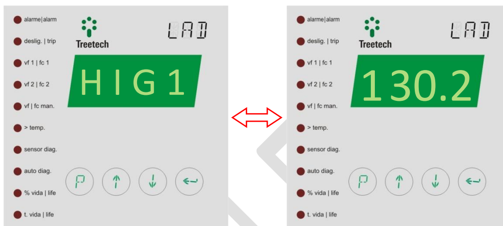
Figure 19: Checking maximum temperatures
