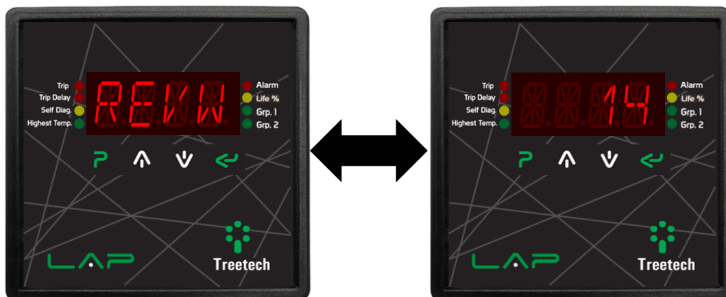
Figure 15 - Display indicating board revision week
