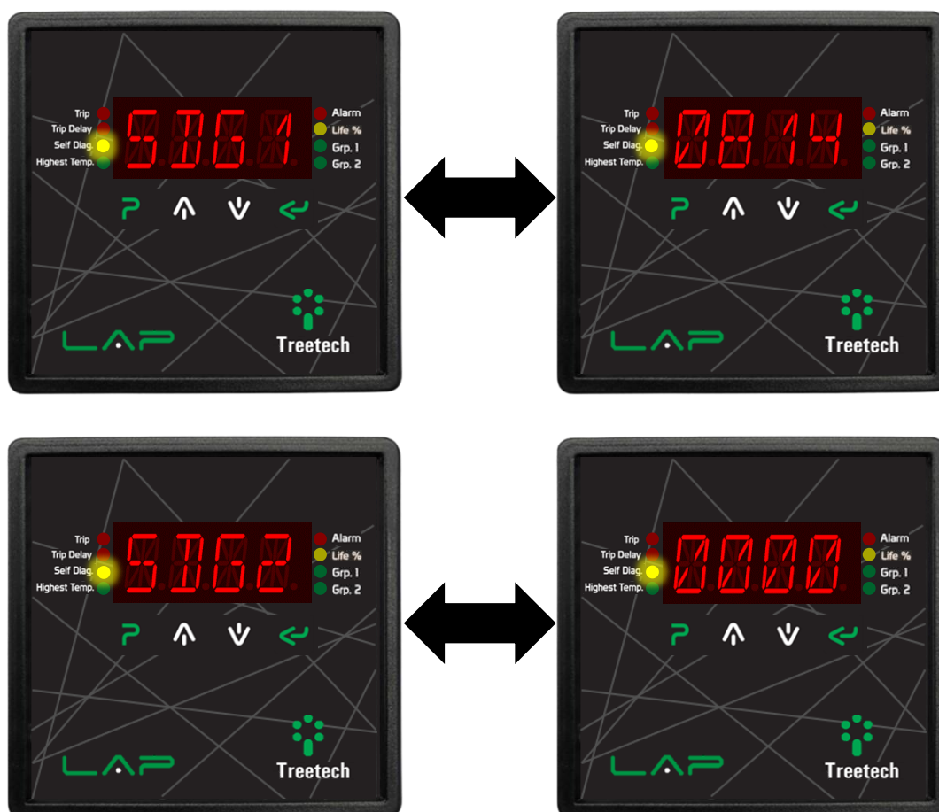
Figure 41 - Self-diagnosis indication on the LAP
