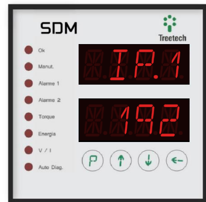
Figure 33 - SDM front panel displaying the IP address for accessing the webpage
