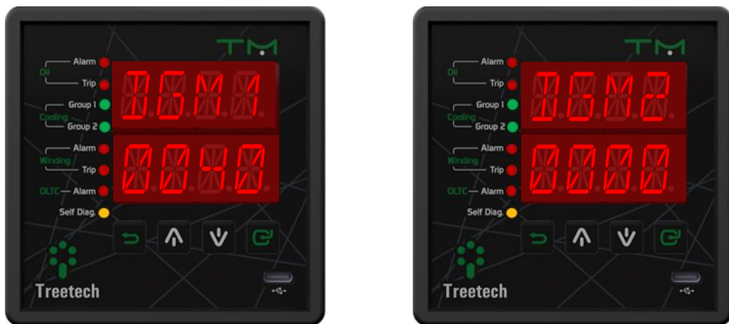
Figure 20 - Querying the self-diagnosis memory
