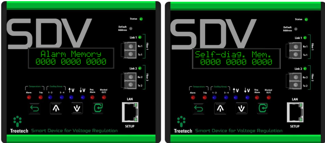
Figure 113 - Alarm memory and self-diagnosis
