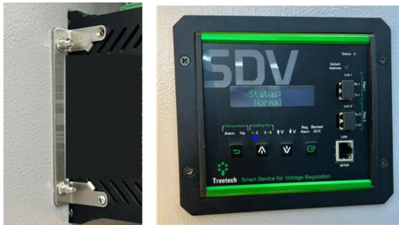
Figure 12 - Panel-mounted equipment with locks and bezel installed
