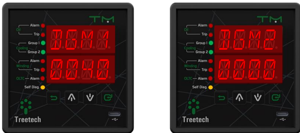
Figure 20 - Querying the self-diagnosis memory
