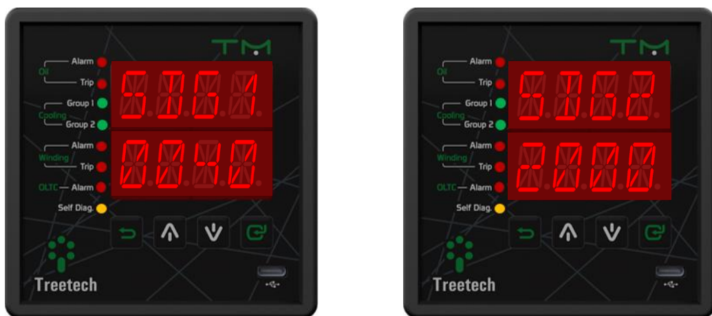
Figure 19 - Indication of self-diagnosis in TM
